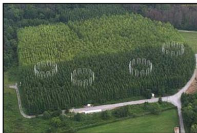
The FACE site consists of five 25 m-diameter rings. FACE apparatus was built around four of the five rings - for a total of 2 elevated (544 ppm) & 3 ambient (391 ppm) rings.
